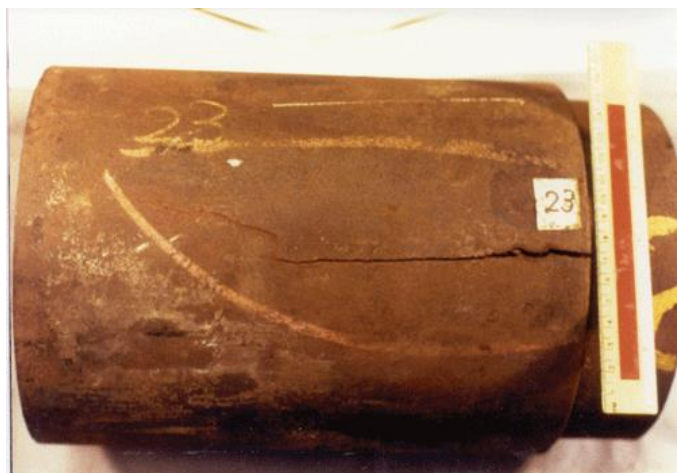
Figure 113: Metal cracking resulting from hydrogen embrittlement 4
