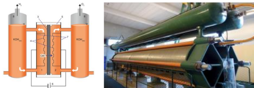
Figure 42: Alkaline cell schematic 3 (left) and real 2.7 MW ch stack 4 (right)
