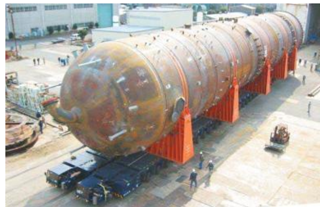
Figure 149: SASOL-Chevron Fischer-Tropsch reactor
