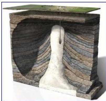
Figure 69: Illustration of a salt cavern 1
