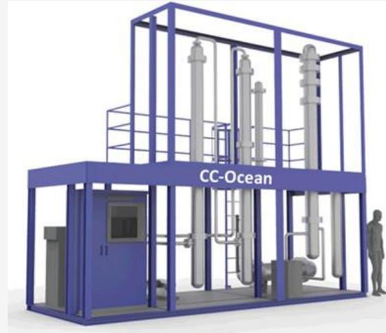
Conceptual drawing of the CO<sub>2</sub> recovery demo plant
