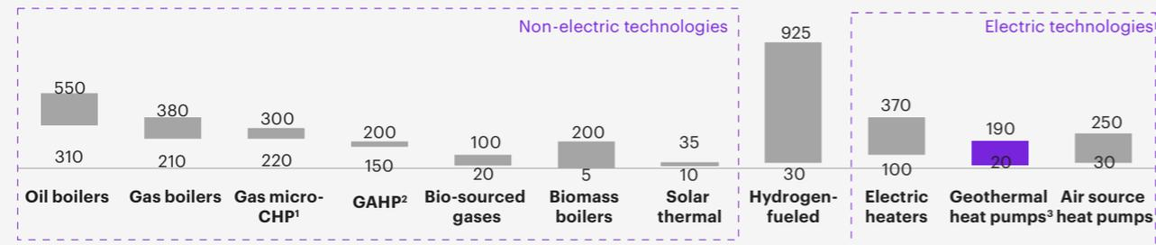
Carbon footprint for power generation technologies (gCO<sub>2</sub>-eq/kWh, 2021)
