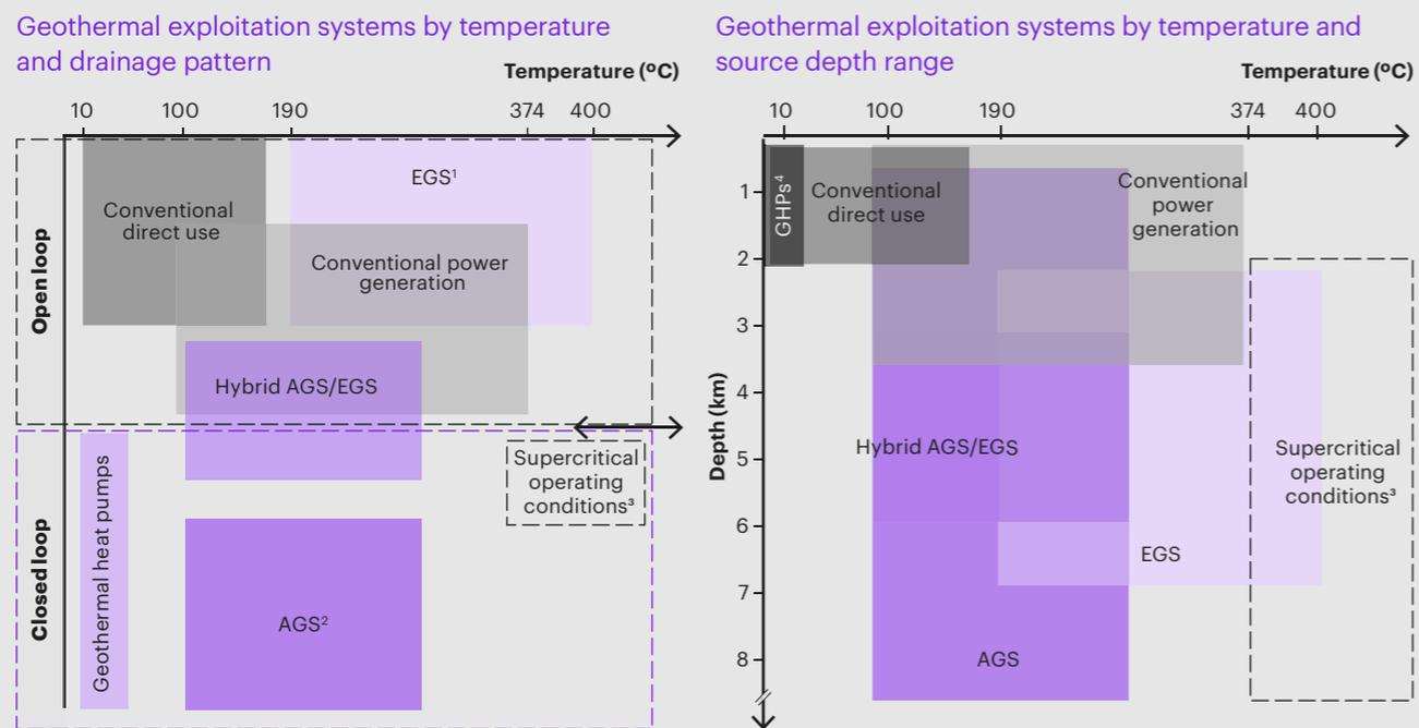
1. Enhanced or engineered geothermal system; 2. Advanced geothermal system;
