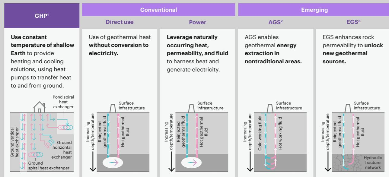
1. Geothermal heat pump; 2. Advanced geothermal system; 3. Engineered geothermal system
