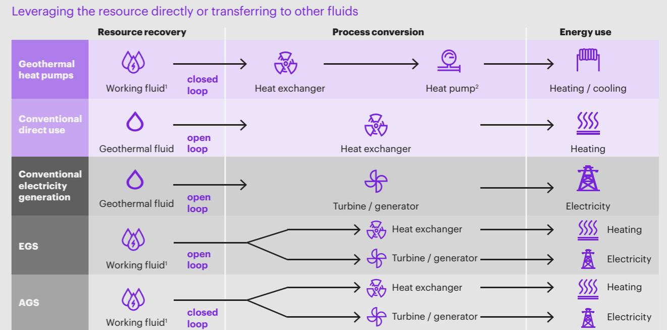
1. Working fluid can be water, an organic compound with a low boiling point, or a mixture depending on environmental regulations, safety considerations, and operating conditions. Working fluid traditionally refers to the fluid circulating through the turbine in a binary-cycle geothermal power plant. In the context of EGS, the term now also applies to the fluid pumped underground to extract heat from the reservoir.; 2. Heat pumps can be operated in reverse to deliver cooling.
