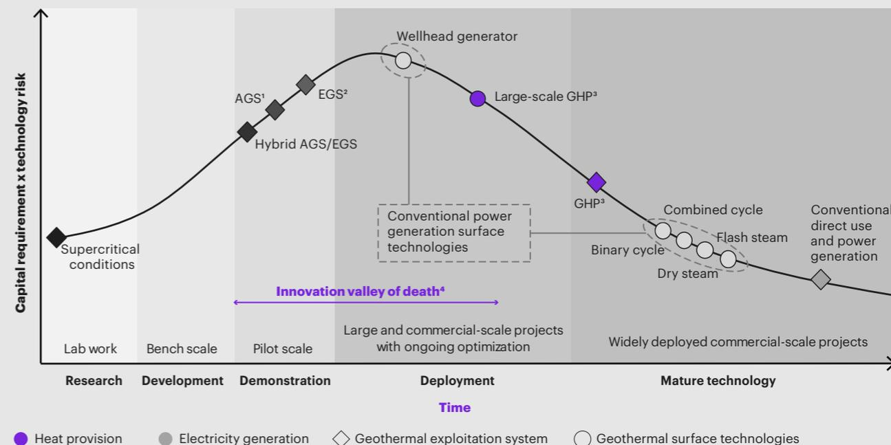
1. Advanced geothermal system; 2. Engineered geothermal system; 3. Geothermal heat pump; 4. Refers to a critical phase in new technology development where the initial momentum and early-stage funding have subsided, but the technology has not yet reached commercialization.
