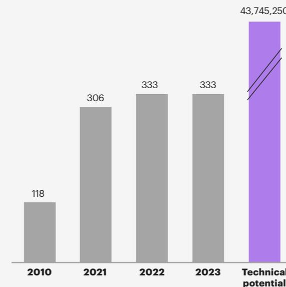
Geothermal electricity generation relative to global technical potential TWh/year, 2010-2023
