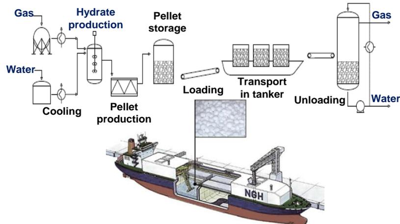
Transportation of natural gas in the form of gas hydrate pellets relies on a kinetic anomaly, known as the self-preservation phenomenon. Under relatively mild pressure and temperature conditions, the formation of a thin ice film around gas-hydrate pellets prevents further destabilization of the gas hydrate. This phenomenon makes it possible to store natural gas in hydrate pellet form far outside its thermodynamic stability field for long periods<sup>2</sup>.
