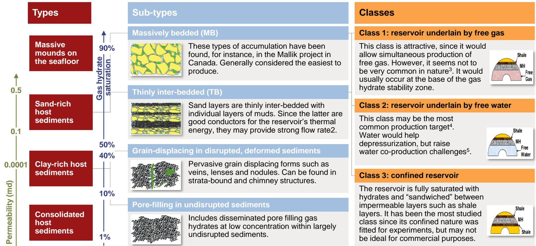
1. Gas hydrates are represented in green. Classes are for sand-rich host sediments only, since the others are less likely to be developed, limiting the need for categorization. Note that Boswell *et al* equally present a Class 4 setting, which describes locations where marine hydrates occur at low saturation (typically <10%) and are dispersed in unconfined coarse materials;
