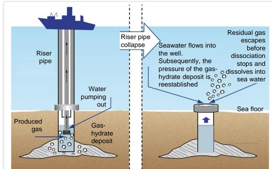
If an accident similar to the 2010 Macondo disaster in the Gulf of Mexico was to happen, seawater would flow into the production well. Therefore, the pressure on the deposit would increase and be restored, and hydrate dissociation – and subsequent gas production – would soon stop.
