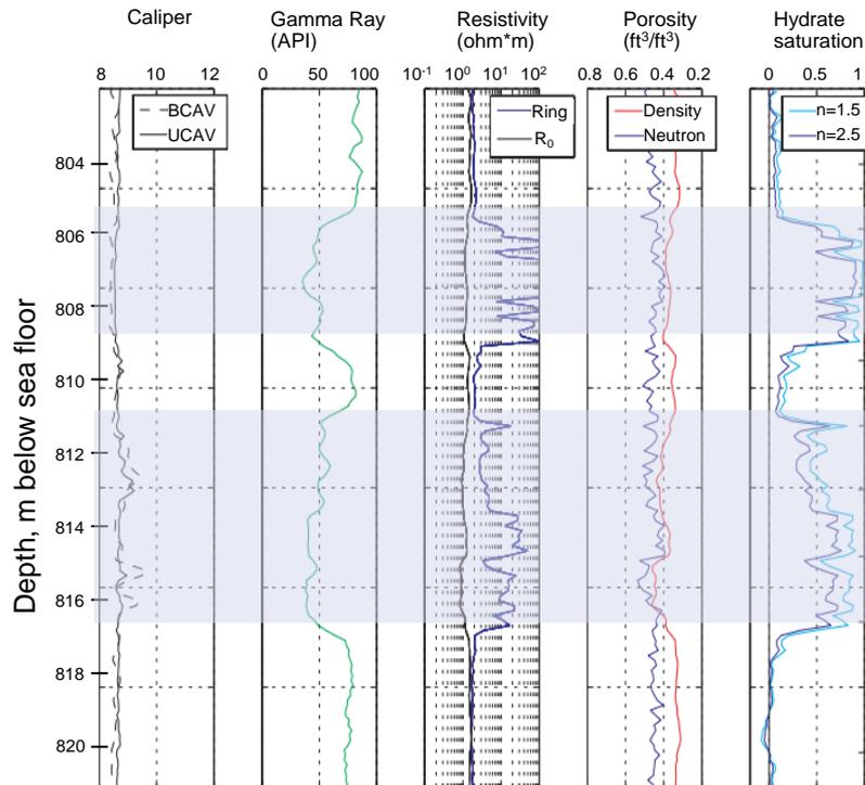
High resistivities are the clearest indications of gas hydrates depicted by pink shading. Estimated hydrate saturation range from 40% to more than 75%
