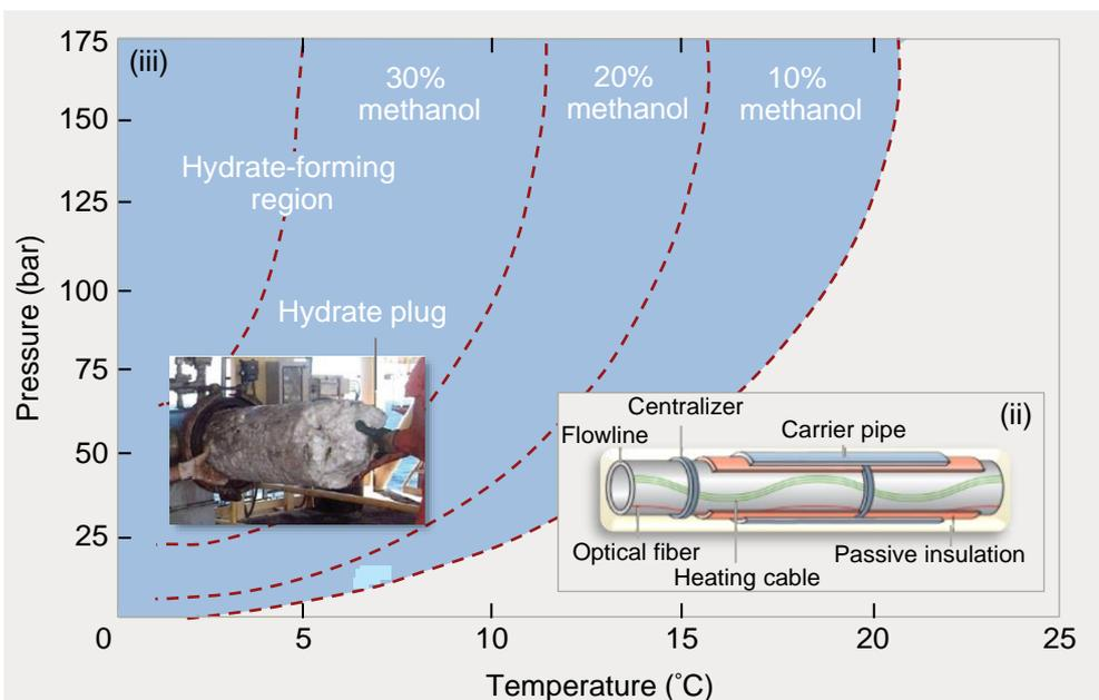
During their path from a deep-water well to the platform and central processing facility, the fluids in a pipeline are subject to temperature and pressure changes. Within the shaded area, it is possible for gas hydrates to form inside and plug the pipeline. Adding chemical inhibitors such as methanol can shift the stability zone to colder temperatures, preventing the formation of hydrate plugs.
