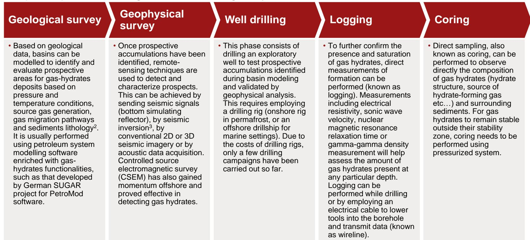
1. Note that the process is not fully sequential. Logging can be performed while drilling, and geophysical survey can use data acquired during previous logging or drilling campaigns; 2. For more information on petroleum system approach, please refer to slides 22 to 26; 3. Seismic inversion consists in extracting quantitative information about reservoir rocks and fluid parameters from seismic data.
