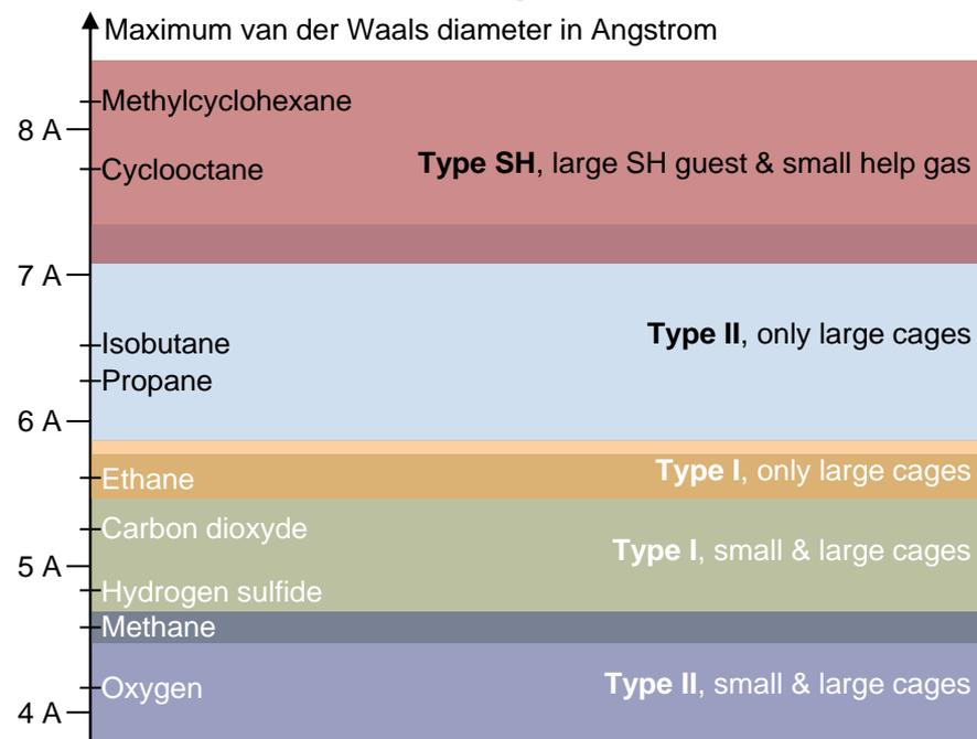
The type of structure formed depends primarily on the size of the enclosed molecule. In nature, most gas-hydrate deposits are Structure I because they are composed of pure methane and do not contain heavier hydrocarbons. Conversely, in oil and gas pipelines, hydrates are mainly Structure II or Structure H, although these are rarer because of the presence of larger hydrocarbons such as propane.
