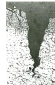
Hydrogen embrittlement occurs at points of stress concentration (hard spots, such as joints) and is expected to be a risk only for high-strength steel (superior to 100 ksi yield strength). Fracture resulting from hydrogen damage happens suddenly without any visible warning signs, and typically affects 2-3% of components
