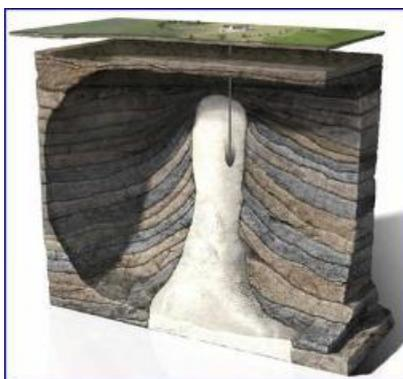
Figure 70: Existing H<sub>2</sub>-caverns in salt domes<sup>2</sup>
