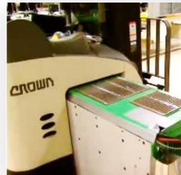
Fuel cell replacing batteries in forklift
