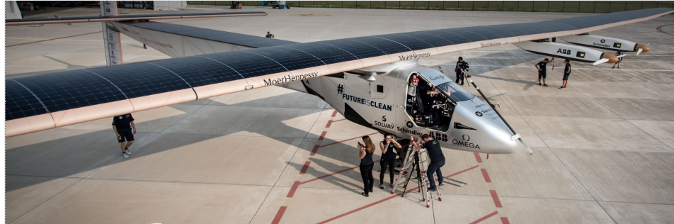
As big as a Boeing 747 (wingspan 72m) but the weight of a car (2,300 kg)
